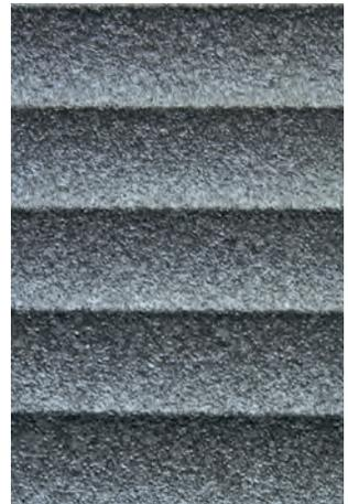
By applying the sintered engobe, surfaces with a metallic structure reminiscent of cast iron are created using metal oxide in the reduction firing technique. Used in the TERRART® façade system, specific impressions and ideas can thus be realised so that unique façade solutions can be found.
